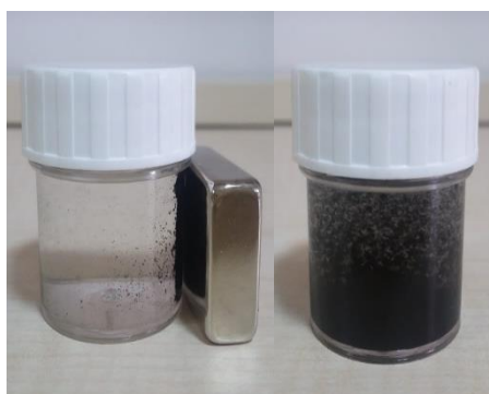
Figure 1. Separation of Fe 3 O 4 -MCCNTs from antibiotic solutions with neodymium magnet
