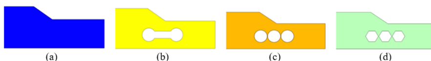
Figure 3. Assumed dimensions of the concept dynamometer (a) and cavity shape (b), hole (c), hexagon (d)
