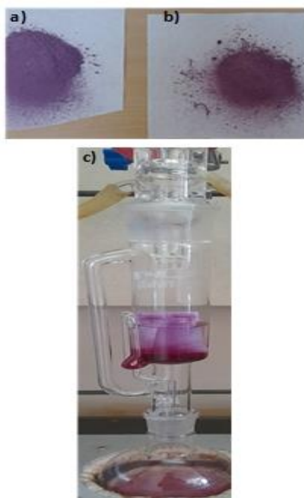
Figure 1. a) Ivy rose extract, b) Velvet red rose extract, c) Production of dyes with the Soxhlet system
