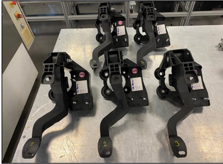
Figure 11. Tested part visuals. No breakage or crack observed.
