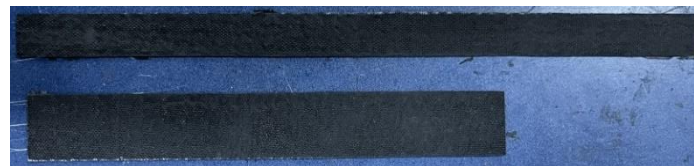
Figure 3. The tensile test specimens of 3D stitched woven composite
