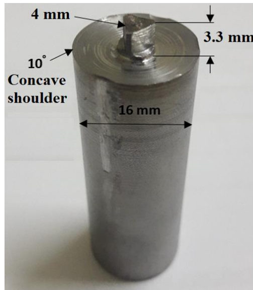
Figure 2. Welding tool used in the FSLW process
