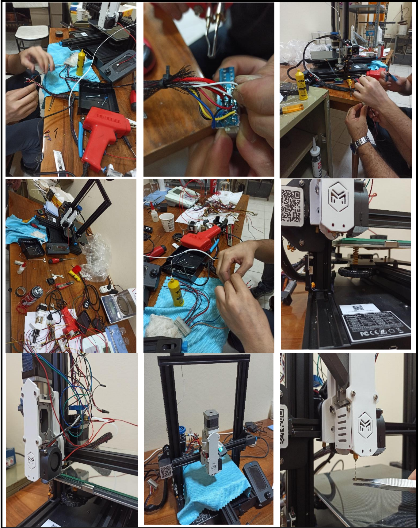
Figure 6. Installation images of the pellet extrusion system on the Creaality Ender 3 V2 three-dimensional printer
