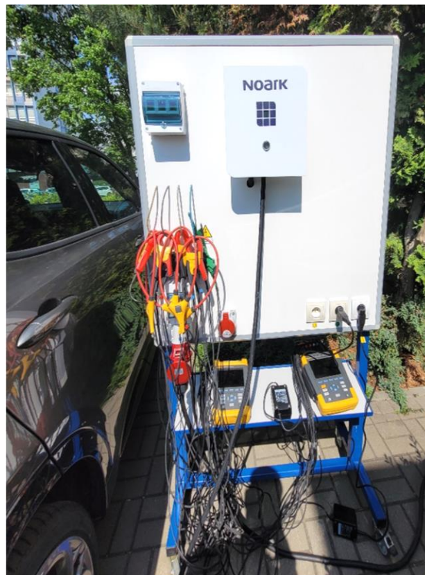
Figure 1. View of test stand. Wallbox in the center, below power and energy analyzers with probes; tested car on the left.
